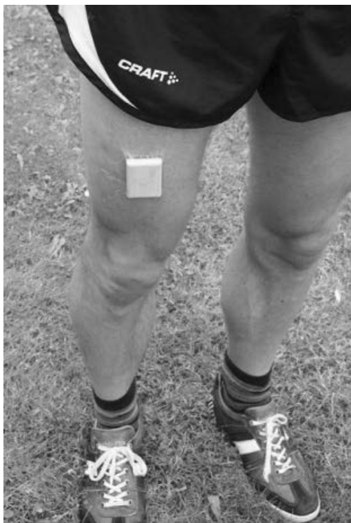
Figure 1.1 Physical activity was objectively measured by a waterproofed accelerometer attached on the thigh during one full week (24 hours/day).
